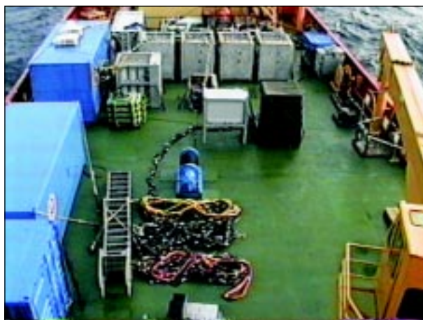
Deck area amidships of the M/V DSESS KELLIE CHOUEST. Two rectangular conex boxes (on left) stored our recompression chambers. Flyaway Mixed Gas System and its five racks are shown at the top. Divers' umbilicals are shown in the middle.
